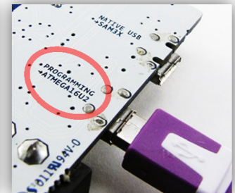
Figure xxx. Arduino Due users should plug the small end of the programming cable into the micro-USB socket labeled "Programming".
