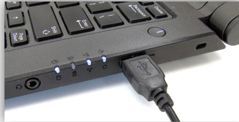
Figure xxx. Plug the USB programming cable into the computer's USB port. Try to use the same port each time you program our development board
