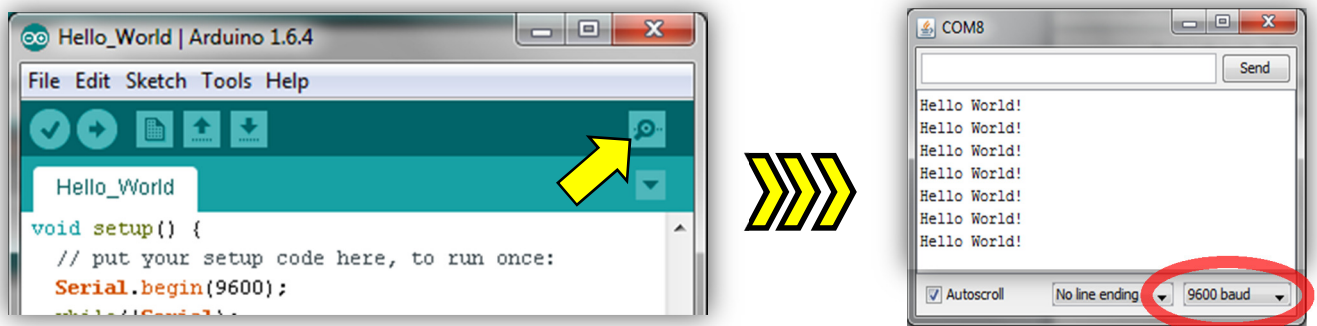
Figure xxx. Open the Serial Monitor to see the printed output of the sketch. Make sure the Serial Monitor is set to a baud rate of 9600.
